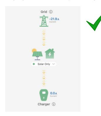
Don't use the Solar Only mode when solar export is low as shown below. Charging will be paused or possibly start and stop continuously due to low export. Solar Assist or Fast Mode recommended to have a stable charge.
